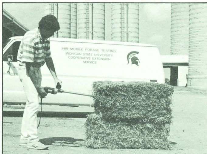
Figure 1. The proper method of sampling a square bale. From the end of the bale, drill in 12 inches near the center at a right angle to the surface.
