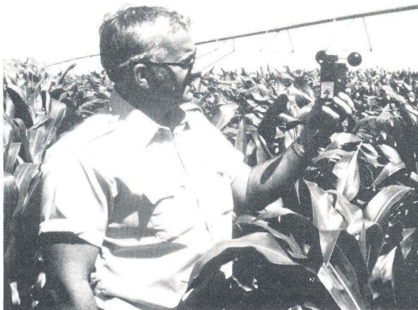
Problems resulting from spray drift can be reduced by monitoring wind.
