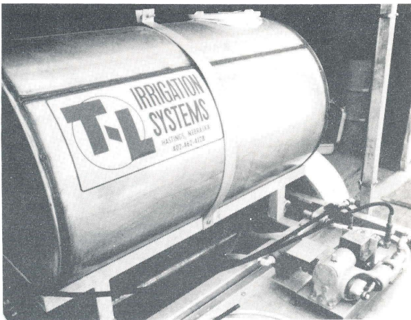
Trailer mounted chemical tank permits use at multiple injection sites.
