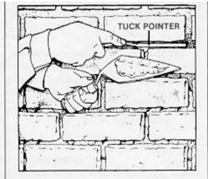
Figure 2. Repair of cracked or crumbling mortar joints is called tuck pointing.
