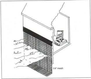
Figure 1. A curtain wall of hardware cloth can prevent rats from burrowing under concrete slabs or foundation walls.
