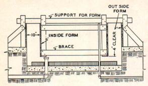
Fig. 5. Step No. 3. The outside forms have been placed for the wall of the tank and the inside forms are supported on the outside forms. Bottom of inside forms should be 4 inches above floor insulation.
