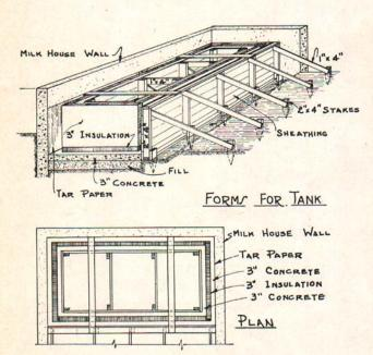
Fig. 6. Another method of setting inside and outside forms for the concrete tank.
