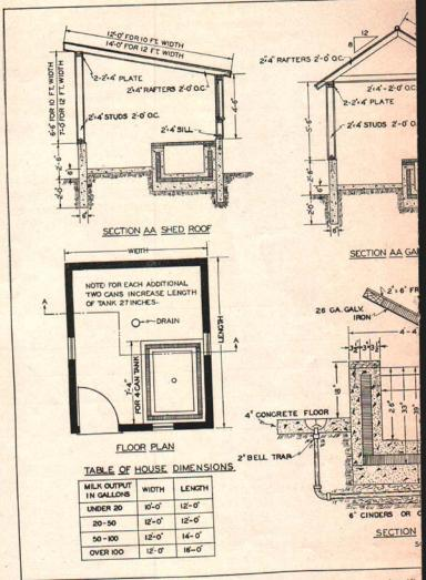
Fig. 1. Details of construction of milk house and cooling tank. (Pro
