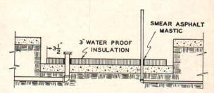
Fig. 3. Step No. 2. Here the 3" water-proof package insulation has been placed on the cement floor. Note that a 3½" space is left all around the insulation for the concrete wall. The insulation should be arranged as shown in Fig. 4 (below).
