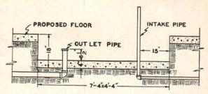
Fig. 2. Step No. 1 shows the excavation for the tank with the concrete sub-floor in place.
