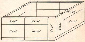
Fig. 8. Method of arranging the insulation for the side walls of a four-can tank.
