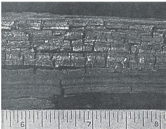
Figure 7.1. Brown rot with characteristic cracks along the grain.
