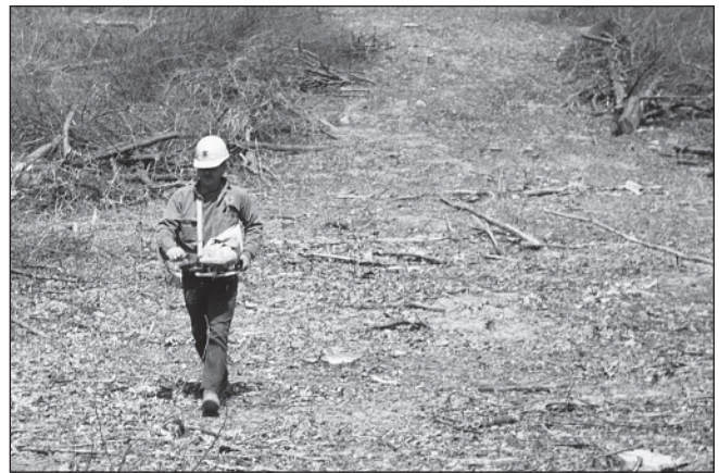
This applicator is using a hand-held pellet applicator sometimes referred to as a belly grinder.
