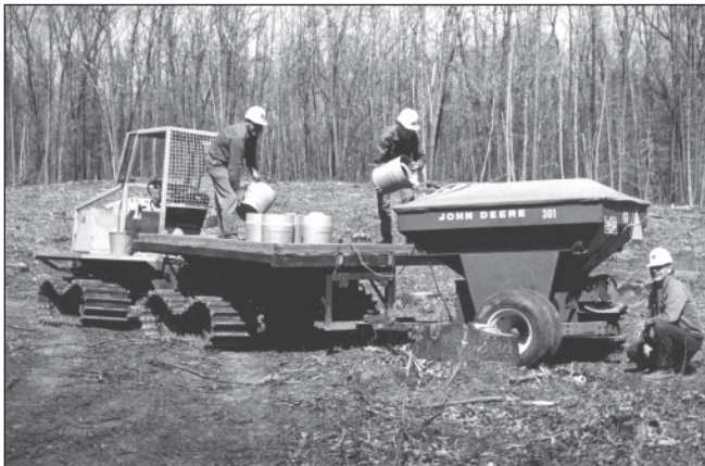
These applicators are loading a granular mechanical spreader. Their hats are good protective clothing although they should also be wearing gloves.
