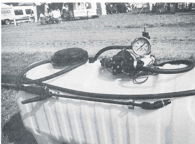
Sprayer tank, wand, pump and gauge.
