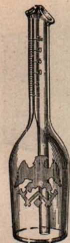
FIG. 17. A skim-milk test bottle on which each subdivision represents .01 of one per cent.
