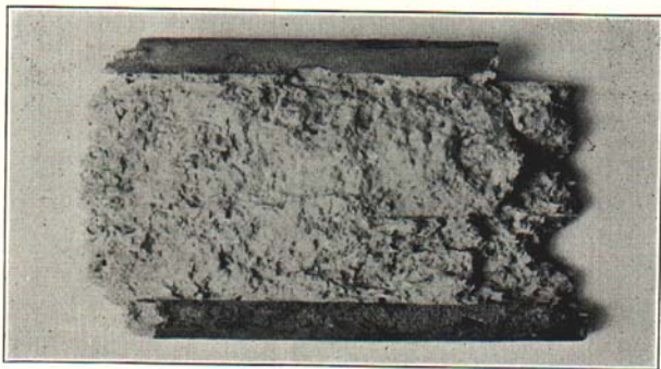
Fig. 11. Piece of wood split open to show inner part reduced to powder.
