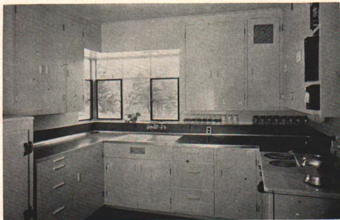
Fig. 27. An example of a U-shaped kitchen arrangement, in which adequate storage and working space are conveniently and compactly grouped.
