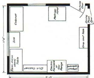
Fig. 30. A broken U-arrangement using portable equipment.
