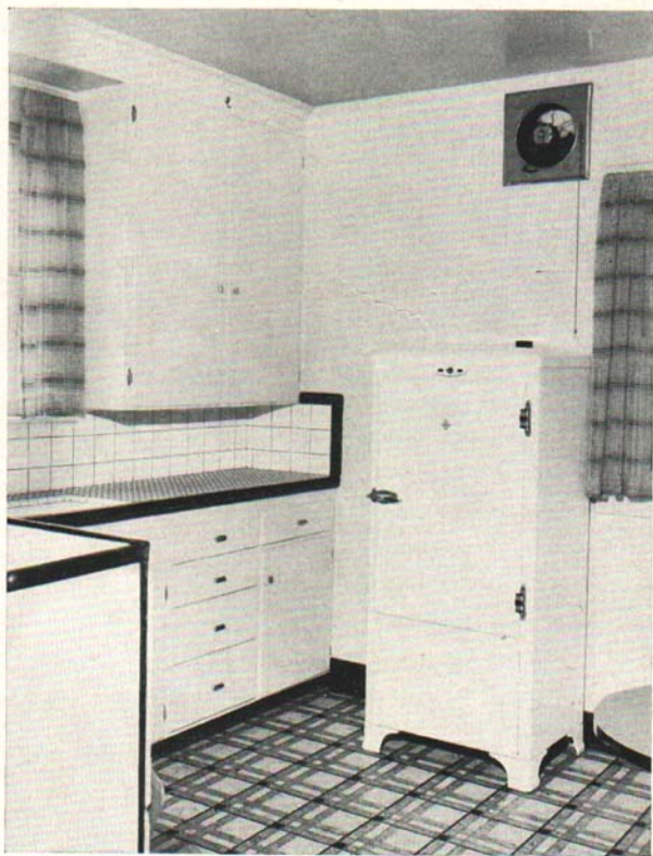
Fig. 1. The two windows provide adequate light and cross-ventilation. The electric fan in the wall above the refrigerator quickly rids the kitchen of undesirable odors. (Another view of the kitchen in Fig. 21.)
