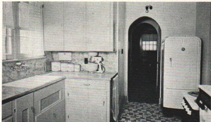
Fig. 20. A broken U-arrangement. The refrigerator and stove are near the mixing cupboard and sink. The dish cupboard is at the left of the sink. This is another view of the kitchen in Fig. 19.
