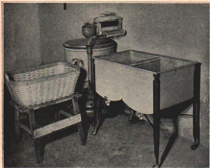
Fig. 1. Equipment for washing including machine, wringer, two portable tubs, basket and stand. Note the drains on the tubs and the wall outlet for attaching the machine. Running water would add to the efficiency of this arrangement.
