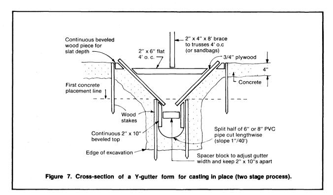
Fresh concrete should be vibrated to fill the space beneath the inner frame, to prevent water leakage from the gutter, and to provide a smooth surface. A semicircular bottom can be constructed by cutting a 6- or 8-in. PVC pipe in half lengthwise and nailing the half-pipe in the bottom of the inner frame.
