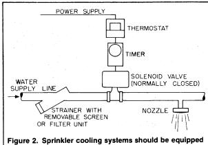
Figure 2. Sprinkler cooling systems should be equipped with a timer-operated solenoid valve, and an in-line sediment filter (strainer).
