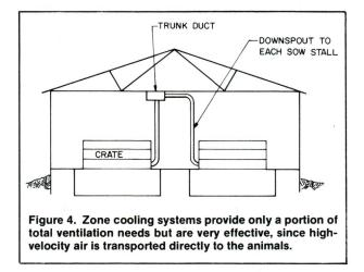
The downspouts should be placed as close as possible to the animals' heads. They should be constructed of nondestructible material and well anchored if within the animal's reach. If the duct opening is too far above the animal, the cooled air mixes with the surrounding air, both reducing its velocity and raising its temperature. Dampers can be used on downspouts to shut off the airflow when crates or pens are empty.
