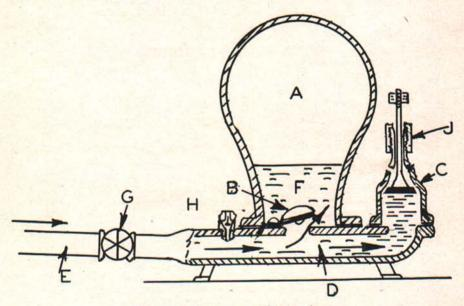
Fig. 2. Hydraulic ram with low base.
