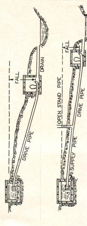
Fig. 4. (upper) The usual arrangement of the drive pipe. (lower) Arrangement of the drive pipe for a distant supply.
