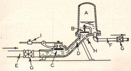
Fig. 1. Hydraulic ram with a high base. (A) air chamber; (B) check valve; (C) outside (impetus) valve; (D) base; (E) drive pipe; (F) delivery pipe; (G) gate valve; (H) air feeder valve; (I) moveable weight for outside valve; (J) adjusting nuts for outside valve.
