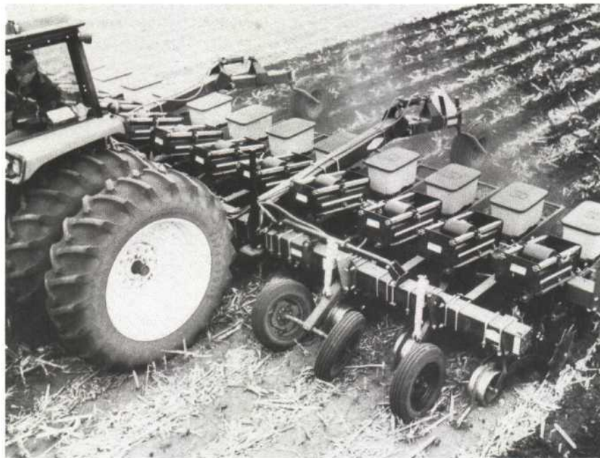
FIGURE 2. Corn being till planted on ridges. Most of the residues from the previous corn crop is located in the valleys where they support both planter and tractor tires. This represents a controlled traffic method which should reduce opportunities for excessively compact soil. Photo — Hiniker Company, Mankato, MN
