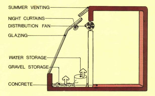
The **isolated gain** system provides for a thermally separated space to collect and store solar radiation which can then be distributed to the living area on demand. An example of an isolated gain design is a greenhouse or sunspace built as a lean-to on the south side of an existing house.
