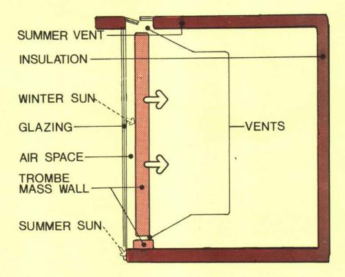
The **indirect gain** concept usually requires a double wall system. A mass wall of stone, concrete or water intercepts solar radiation entering through the south glazing.
