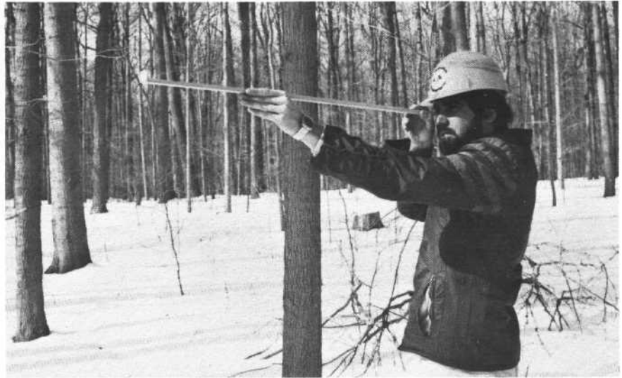
Fig. 4. To estimate basal area using an angle gauge, the observer turns a complete circle over the sampling point and counts the total number of trees larger than the width of the block.
