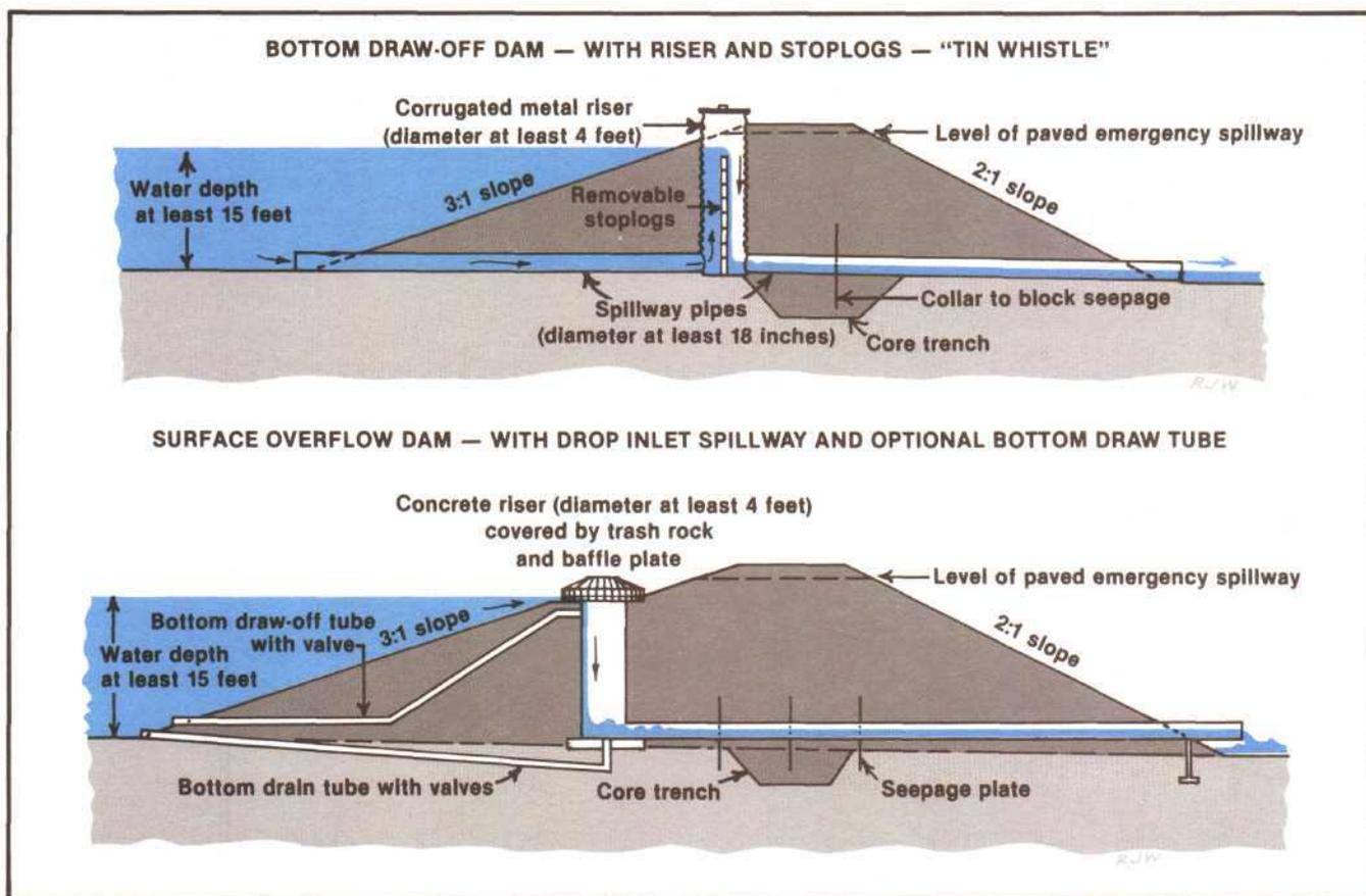
Two common types of outlet structures for dams that form fish ponds. Riser-and-stoplog construction is the simplest design that allows controlled bottom draw-off. A drop-inlet spillway can accommodate greater variation of flow. It is needed where run-off from large land area supplies the pond and where sudden high water is expected.
