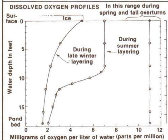
Dissolved oxygen at different depths in the same pond, as affected by the wind mixing and thermal/density layering shown in the figure on page 20.
