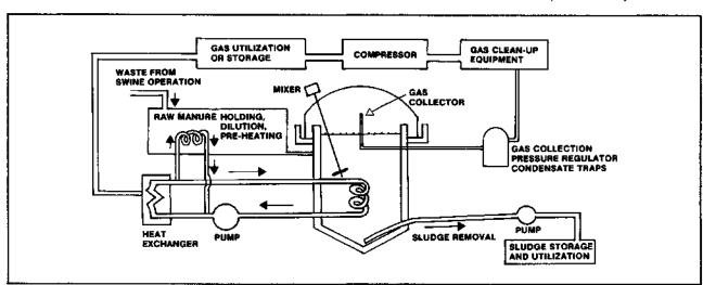
Figure 1. Anaerobic digester.
