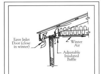
Figure 13. Adjustable slot inlet design for removing air from the attic in winter and from under eaves in summer.
