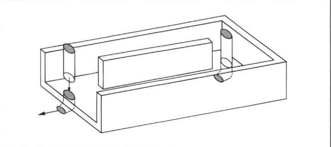
Figure 11. Flat bottom drain gutter with plug at each end.
