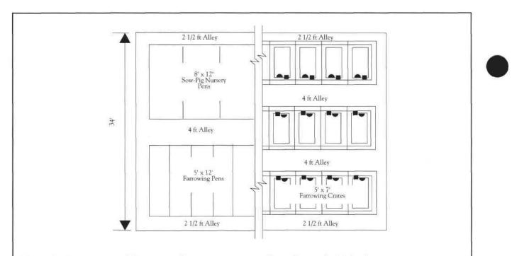
Figure 1. Arrangement of three rows of crates or two rows of pens in a typical dairy barn.
