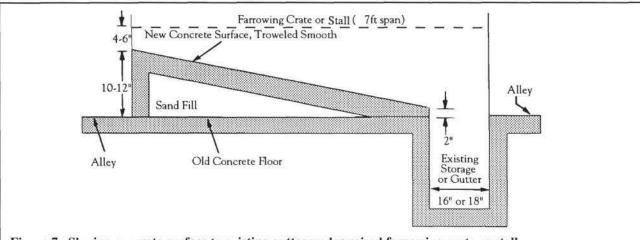
Figure 7. Sloping concrete surface to existing gutter under raised farrowing crate or stall.
