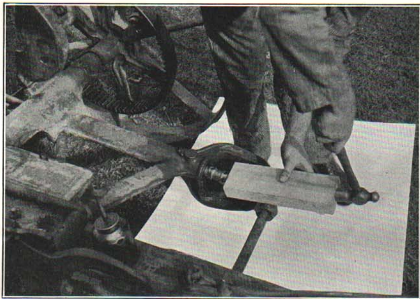
Fig. 7. Replacing lower crankshaft bearing. Fly-wheel removed.
