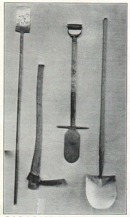
Fig. 8. Planting Tools. Left to Right-Michigan planting bar (inverted in photograph) Grub Hoe-Howard Planting tool-Shovel, common round pointed long handled style.
