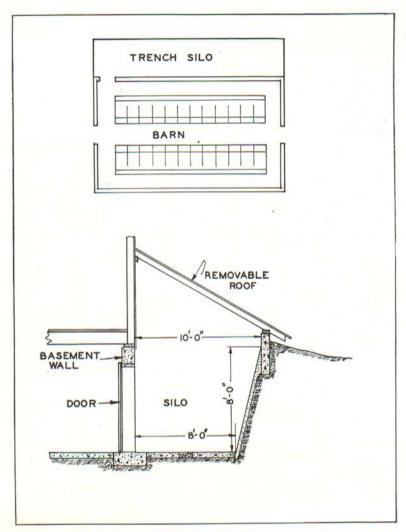
Fig. 5. A convenient location for a trench silo.
