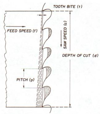
Fig. 1—Cutting Action of band saw.
