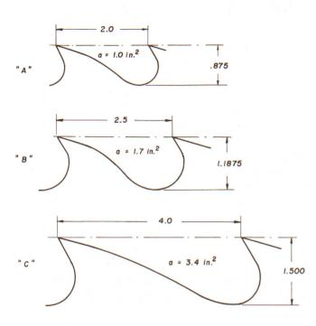
Fig. 6—Gullet space and tooth dimensions of selected band saws "A", "B", and "C".
