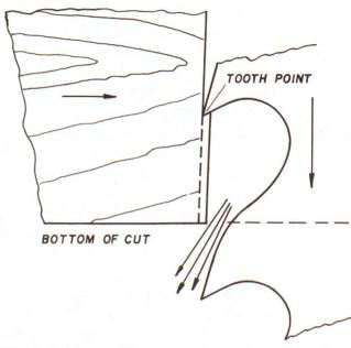
Fig. 4—Schematic illustration of saw dust release from gullet before tooth point reaches bottom of cut. From Quelch (2).
