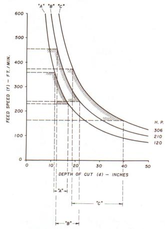
Fig. 5—Operating characteristics of selected band saws "A", "B", and "C".
