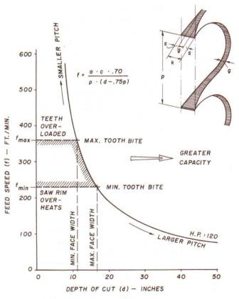
Fig. 3-Operating characteristic of band saw "A".
