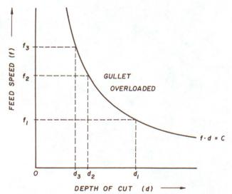
Fig. 2—Characteristic curve of saw indicates relationship between feed speed and depth of cut at gullet capacity.
