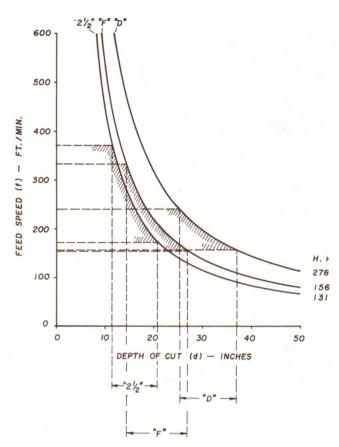
Fig. 7—Operating characteristics of three standard inserted tooth circular saws.
