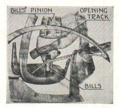
Fig. 7. Step 2 in the Tying Process.
