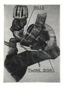
Fig. 6. Step 1 in the Tying Process.
