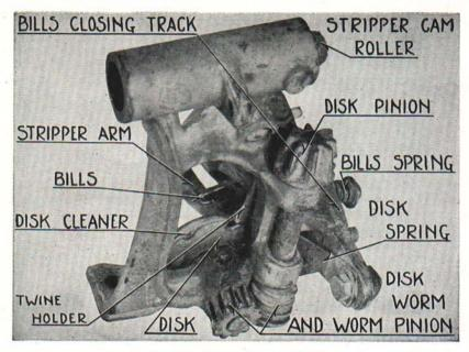
Fig. 13. Deere Knotter Head.
