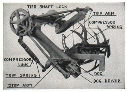
Fig. 3. McCormick or I. H. C. Model M Binder Head.
