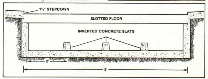
Figure 2. Cross-section of an underslat flushed gutter with dividers.
