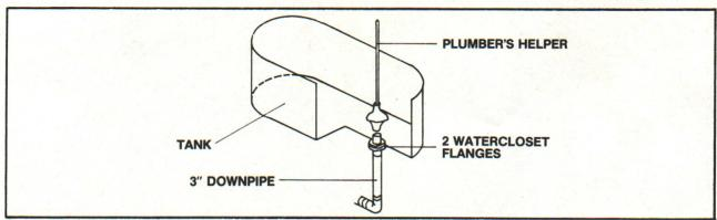
Figure 6. Cut-away view of manual flush tank.
