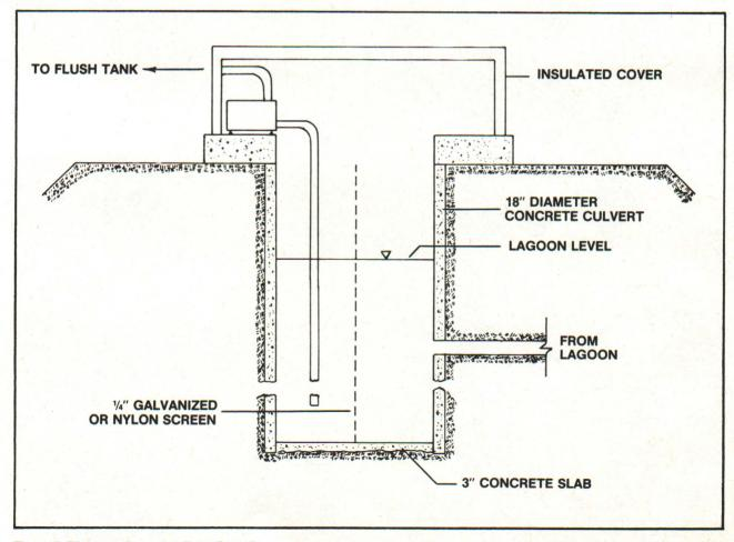
Figure 8. Diagram of a wet-well configuration.
