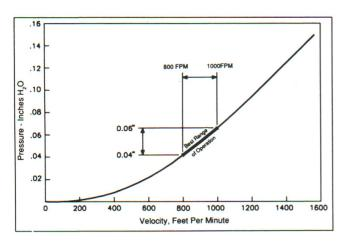
Figure 6. Air intake velocity and static pressure relationship.
