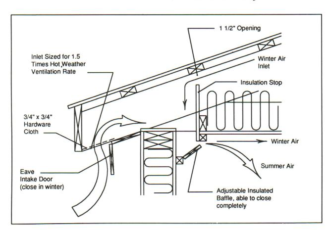
Figure 7. Typical eave and baffled slot intake. Source: Midwest Plan Service, MWPS-32, Mechanical Ventilating Systems Handbook.
