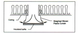
Figure 9. Gravity curtain inlet. The curtain is weighted in order to restrict the air inlet size and thus maintain a high incoming air velocity to promote mixing and distribution of fresh air.
