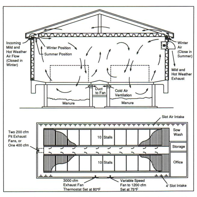
Figure 2. A type of negative pressure (exhaust) ventilation system with pit ventilation. The cold weather ventilation rate is exhausted through properly sized openings into the under-aisle duct.
