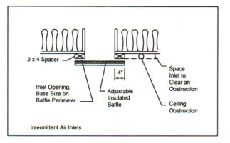
Figure 8. Baffled air inlets for "across-the-ceiling" airflow. Do not mount pipes or lights within 4 ft. of inlets-a smooth ceiling prevents cold air from being deflected down onto animals.
