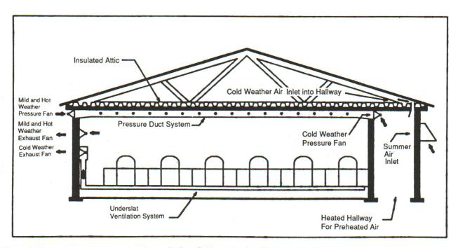
Figure 4. Neutral pressure, or push-pull ventilation. Cold weather ventilation is distributed through the pressurized duct while mild and hot weather ventilation is typically operated as a negative pressure system.
