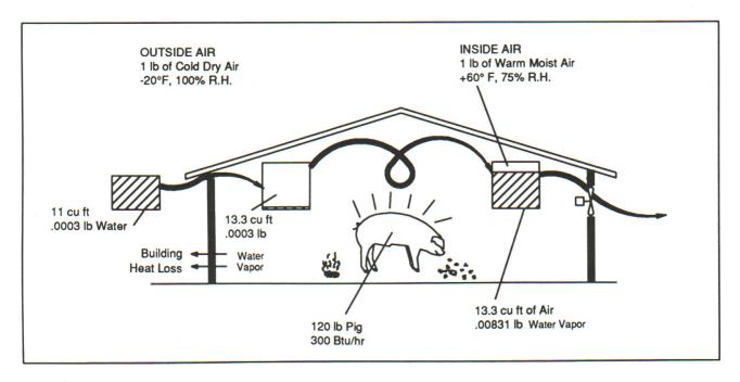
Figure 1. Winter ventilation in a controlled environment. Source: MWPS-32, Midwest Plan Service Mechanical Ventilating Systems Handbook.
