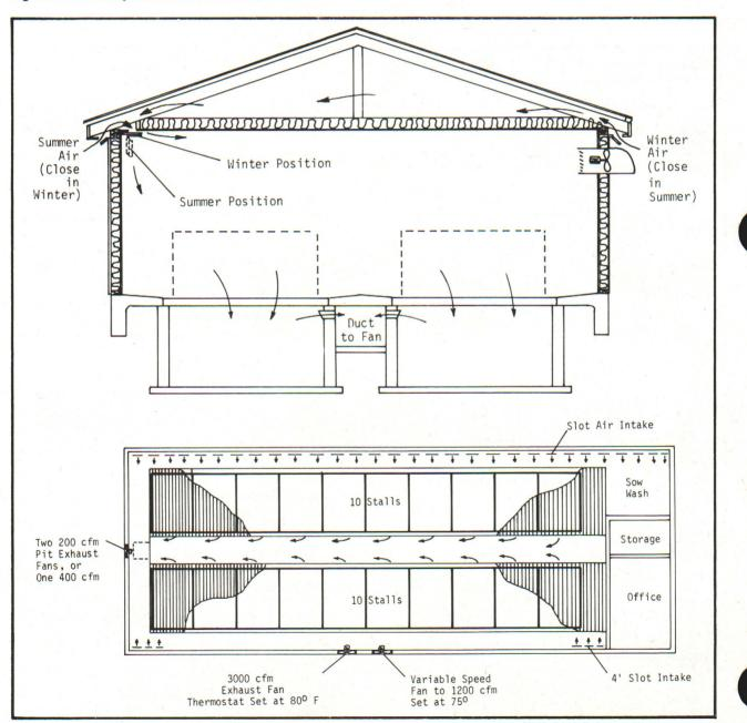
Figure 5. One type of negative pressure (exhaust) ventilation system with pit ventilation.
