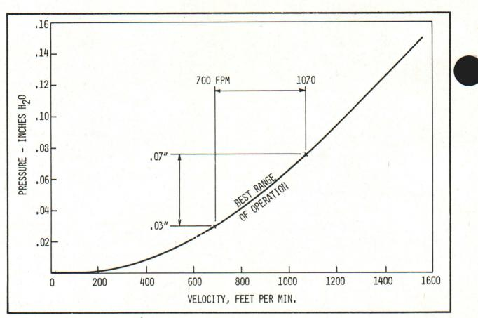
Figure 6. Air intake velocity and static pressure relationship.
