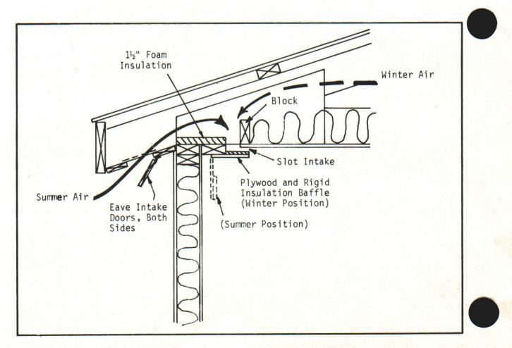
Figure 7. Typical eave and baffled slot intake. Source: Midwest Plan Service.
