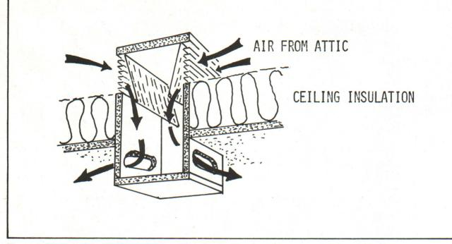
Figure 8. Rectangular ceiling area intake with self-adjusting damper.
