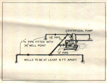
Fig. 12.—A number of shallow wells 15 to 20 ft. deep may be connected together and operated with one pump.
