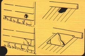
COVER MOUSE HOLES. **CRACKS, AND EXTERIOR** WALL OPENINGS WITH **METAL PATCHES**
