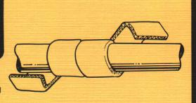
WRAP HOT WATER PIPES **INSULATION STRIPS WITH** 2" BLANKET.
