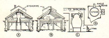
A building of this size can be heated conveniently with a stove or small furnace. The stove may be located in the head house and sometimes the smoke pipe is extended through the sash house just below the sash as shown at A and B in the above drawing. In using this method of heating, precautions should be taken to prevent leakage of smoke into the house. Stove pipe made in six- or eight-foot lengths and the joints soldered is sometimes used.
