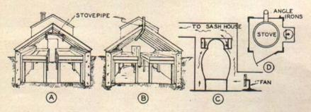
A building of this size can be heated conveniently with a stove or small furnace. The stove may be located in the head house and sometimes the smoke pipe is extended through the sash house just below the sash as shown at A and B in the above drawing. In using this method of heating, precautions should be taken to prevent leakage of smoke into the house. Stove pipe made in six or eight foot lengths and the joints soldered are sometimes used.
