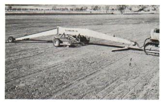
Figure 3. Land level only recently tilled soil where no crop residues or trash are exposed. A minimum of three treatments, each in a different direction, is recommended. This should be repeated one or two years later because the transported soil material will settle.
