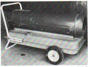
Figure 3. Temporary-type portable heater using fuel oil as the energy source. Blower and controls connect to 115 volt outlet.
