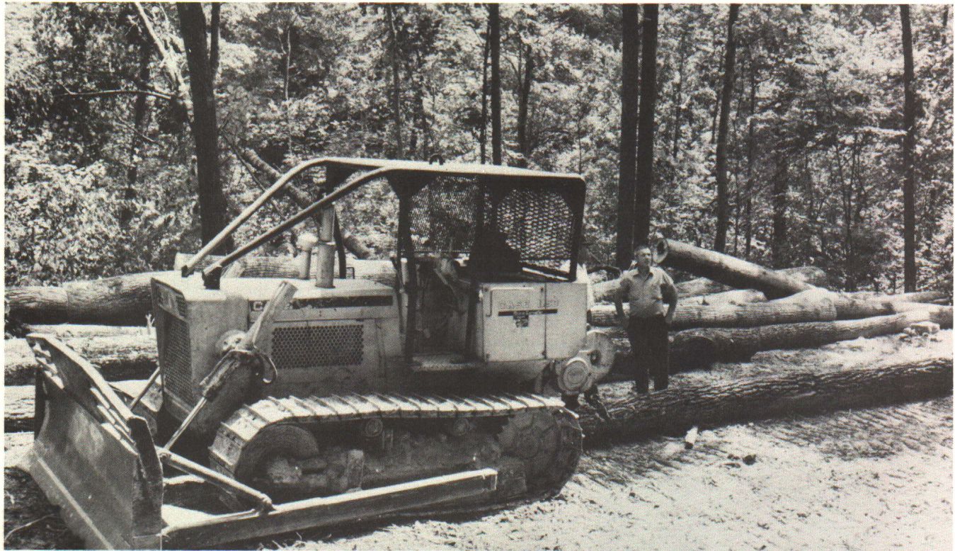
Appropriate equipment is necessary when large amounts of timber are to be harvested. A small bulldozer is well suited for constructing logging trails and skidding logs.
