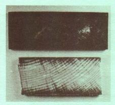
Fig. 12. Adequate and inadequate penetration in two ponderosa pine 2-in. planks cut at the center. A chemical indicator shows copper in CCA-treated wood.
