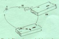
Fig. 4. Stages in spread of decay. Spores (S) are produced in fruiting body (FB) growing on decayed wood. Spores are blown to moist wood and germinate (GS). Wood decays (DW). When wood is heavily rotted, fruiting bodies appear (FB).
