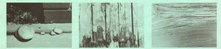
Fig. 5. (Left) Fruiting body resembling a mushroom growing from wood that appears sound on the surface but is decayed within. Fig. 6. (Center) Deck boards decayed by brown rot. Fig. 7. (Right) White rotted wood.
