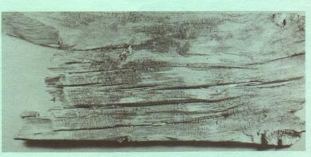
Fig. 8. Board surface destroyed by soft rot. Note small cross checks.
