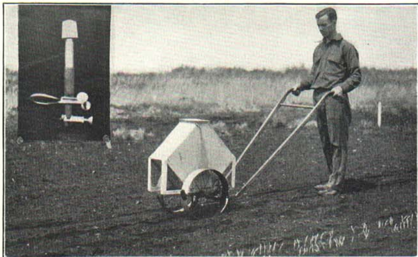
Fig. 14. A home-made distributor for corrosive sublimate treatment for maggot control. The tank attaches to a wheel hoe frame and is of galvanized sheet iron reinforced with angle iron, the inner surface of the tank being covered with asphaltum paint. Dimensions of tank 20 x 20 x 8 inches, with one edge removed to give an 8 x 8 inch base, and the opposite edge removed to give a 6 x 8 inch opening in top. Capacity of tank 12 gallons, sufficiently large for treatment of a row 50 to 60 rods long. The distributing pipe ends in a piece of rubber tubing on which is attached a screw clamp by which the flow is regulated. A pinch clamp is used to close the rubber tubing when flow is not desired. The distributing pipe must be in line with the axles of the wheels and the lower end in plain view of the operator so that the flow can be directed on the onion row. Inset shows distributing pipe with rubber tubing and clamps attached. Three-inch sheet iron rims on wheels facilitate the handling of the machine while a cheese-cloth strainer prevents clogging of the distributing tube.
