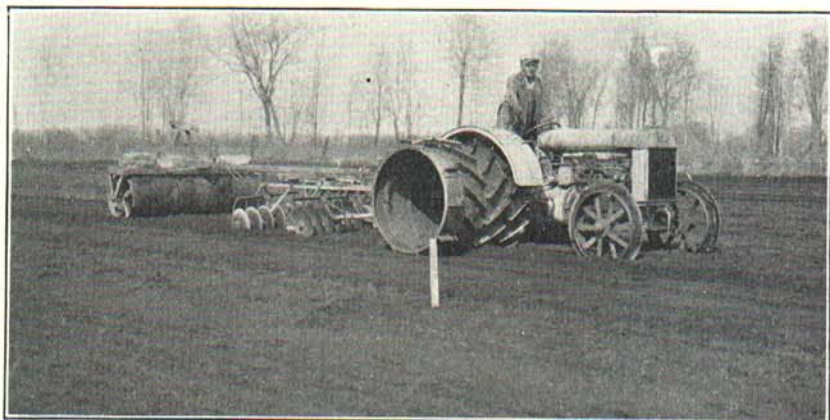
Fig. 8. The double-disc and roller are important in the preparation of the seed bed. On this rather wet muck, the farmer took no chances on having his tractor mired, as can be seen from the extensions on the tractor wheels. On a drier muck, a heavier roller, or cultipacker and float, would have given more satisfactory results.
