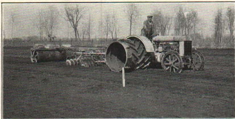
Figure 8.—The double-disc and roller are important in the preparation of the seedbed. On this rather wet muck, the farmer took no chances on having his tractor mired, as can be seen from the extensions on the tractor wheels. On a drier muck, a heavier roller, or cultipacker and float, would have given more satisfactory results.
