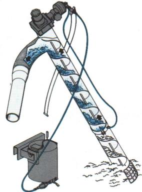
Fig. 3. Commercially available equipment for metering chemical into auger conveyor where it is mixed with seed before going into drillbox or holding container.
