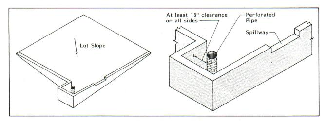
Figure 3. Setting in corner of lot. Settling basins can sometimes be located within a larger lot, if out of main animal traffic routes. Note the emergency overflow for larger storms. Reproduced with permission from: *Livestock Waste Facilities Handbook*, MWPS-18, 2nd Edition, 1985(c) Midwest Plan Service, Ames, IA 50011-3080.
