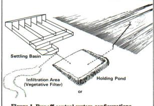
Figure 1. Runoff control system configurations.
