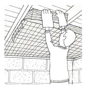
Start at a wall at one end of the joists and work out. Staple the wire to the bottom of the joists, and at right angles to them. Slide batts in on top of the wire. Work with short sections of wire and batts so that it won't be too difficult to get the insulation in place. Plan sections to begin and end at obstructions such as cross bracing.
