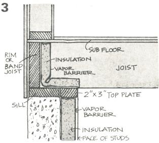
Install another small piece of insulation above the furring and against the sill to insulate the sill and band joist.
