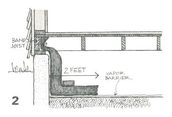
**Drawing 2:** Where the joists run parallel to the wall, you don't need the short pieces of insulation, just install the wall and perimeter insulation by nailing the top of each strip to the Band Joist, using the 1/2" X 1-1/2" nailers.
