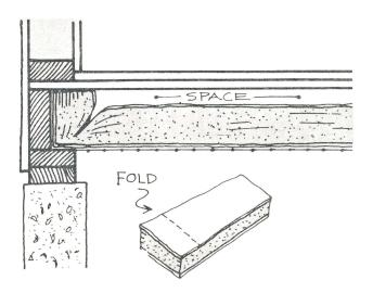
Buy insulation with a vapor barrier, and install the vapor barrier facing up (next to the warm side) leaving an air space between the vapor barrier and the floor. Get foil-faced insulation if you can; it will make the air space insulate better. Be sure that ends of batts fit snugly up against the bottom of the floor to prevent loss of heat up end. Don't block combustion air openings for furnaces.
