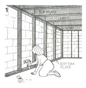
Nail the bottom plate to the floor at the base of the wall with a hammer and concrete nails. Install studs 16 or 24 inches apart after the top plate is nailed to the joists above. (Where the wall runs parallel to the joists, nail the top plate to the tops of the studs, and fasten the studs to the wall.)
