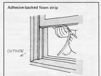
Install adhesive backed foam, on all types of windows, only where there is no friction. On double-hung windows, this is only on the bottom (as shown) and top rails. Other types of windows can use foam strips in many more places.
