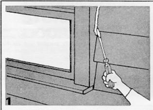
Before applying caulking compound, clean area of paint build-up, dirt, or deteriorated caulk with solvent and putty knife or large screwdriver.
