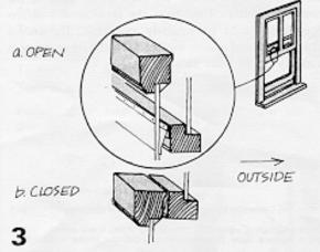
Then attach a strip the full width of the window to the upper sash bottom rail. Countersink the nails slightly so they won't catch on the lower sash top rail.
