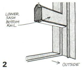
Install strips the full width of the sash on the bottom of the lower sash bottom rail and the top of the upper sash top rail.
