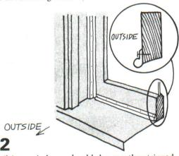
tilting windows should be weatherstripped with the vinyl nailed to the window casing so that, as the window shuts, it compresses the roll.
