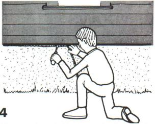
Fill extra wide cracks like those at the sills (where the house meets the foundation) with oakum, glass fiber insulation strips, etc.)
