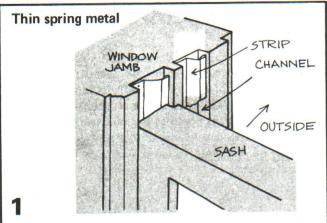
Install by moving sash to the open position and sliding strip in between the sash and the channel. Tack in place into the casing. Do not cover the pulleys in the upper channels.
