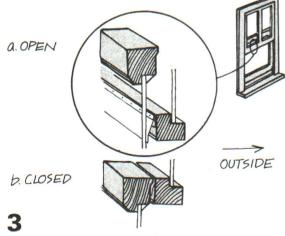
Then attach a strip the full width of the window to the upper sash bottom rail. Countersink the nails slightly so they won't catch on the lower sash top rail.
