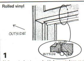
Nail on vinyl strips on double-hung windows as shown. A sliding window is much the same and can be treated as a double-hung window turned on its side. Casement and
