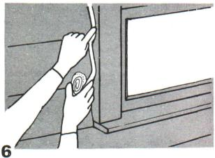
Caulking compound also comes in rope form. Unwind it and force it into cracks with your fingers. You can fill extra long cracks easily this way.
