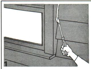
Before applying caulking compound, clean area of paint build-up, dirt, or deteriorated caulk with solvent and putty knife or large screwdriver.
