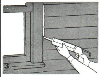
A wide bead may be necessary to make sure caulk adheres to both sides.
