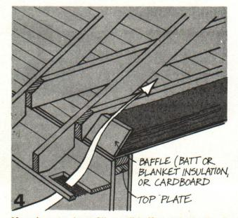
If you're using loose fill, install baffles at the inside of the eave vents so that the insulation won't block the flow of air from the vents into the attic. Be sure that insulation extends out far enough to cover the top plate.
