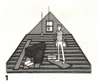
Install temporary flooring and lights. Keep insulation in wrappers until you are ready to install. It comes wrapped in a compressed state and expands when the wrappers are removed.
