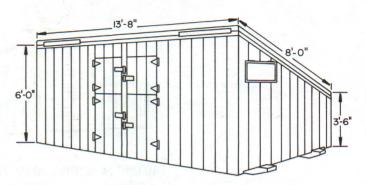
**TWO-SECTION PORTABLE HOG COT 726-CI-17—1 sheet, free** This portable building  $8' \times 14'$  is designed for housing sows and litters on the range. Pig fenders are shown and an electric corner brooder. Doors on all four sides allow good summer ventilation.
