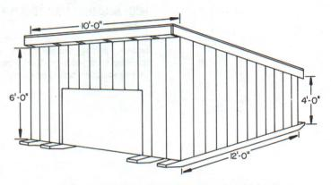
10'  $\times$  12' SHED ROOF HOG HOUSE 726-Cl-20—1 sheet, free This portable range building can house 8 to 12 hogs on pasture. It is on skids so it can be moved around from field to field or brought into a feed lot. Wood frame construction is used and a plank floor. A list of materials is included.
