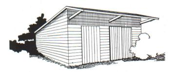
**EXPANDABLE HORSE STABLE 722-CI-16—4 sheets, \$2.00** This expandable horse barn starts out as a  $12' \times 20'$  unit with one box stall and storage for tack, grain, hay and bedding.
