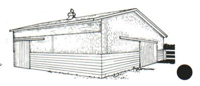
HORSE BARN-POLE CONSTRUCTION 722-Cl-14—4 sheets, \$2.00 This 24'  $\times$  24' pole barn has two 12'  $\times$  12' box stalls that provide ample space for foaling or for large horses. Tack room can be heated, if desired, and there are storage areas for grain, feed and bedding.
