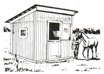
**PORTABLE STABLE FOR A HORSE 6082–2 sheets, \$2.00** This 10'  $\times$  12' portable one-horse stable is planned for economical use of materials with a minimum of waste. It is of wood construction with a corrugated aluminum or galvanized steel and translucent plastic roof.
